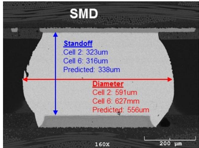
Figure 9: Cross-section of typical SMD solder-joint after mounting to PCB.
