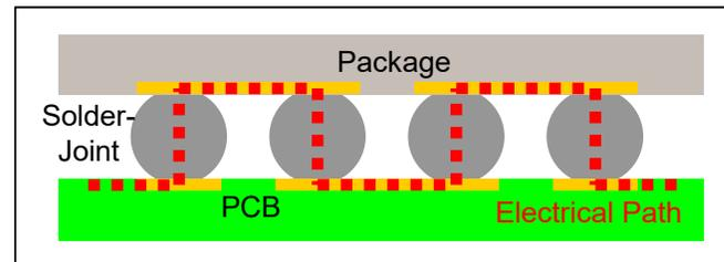
**Figure 2:** A daisy-chain connection representation between package substrate bottom metal and printed circuit board top metal. The red dashed line illustrates the electrical path.
