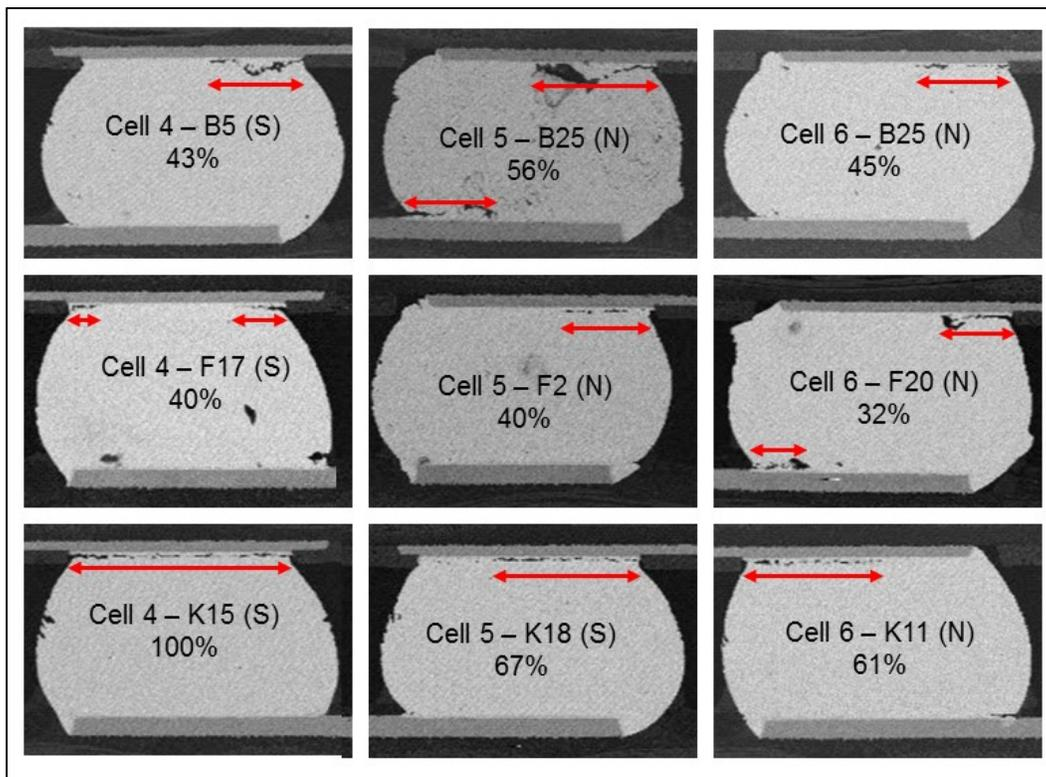
**Figure 14:** Solder-joints with most advanced crack growth after 3000 cycles from Cells 4-6. Pad type is noted parenthetically.
