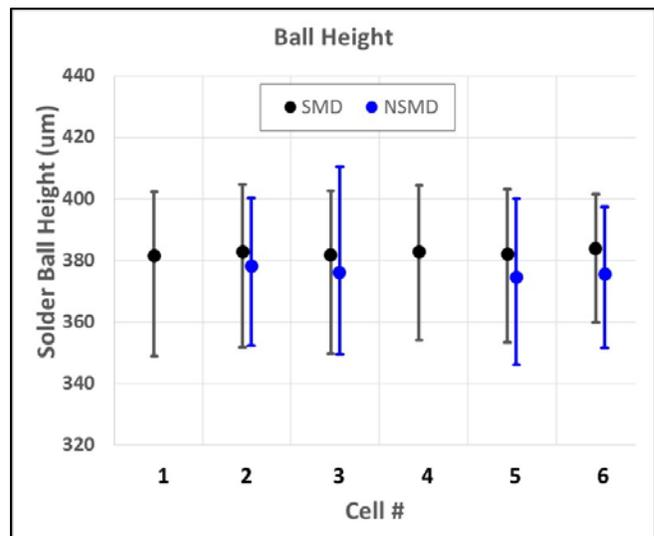
Figure 6: Ball height measurement by RVSI scanner. Error bars represent the data range.
