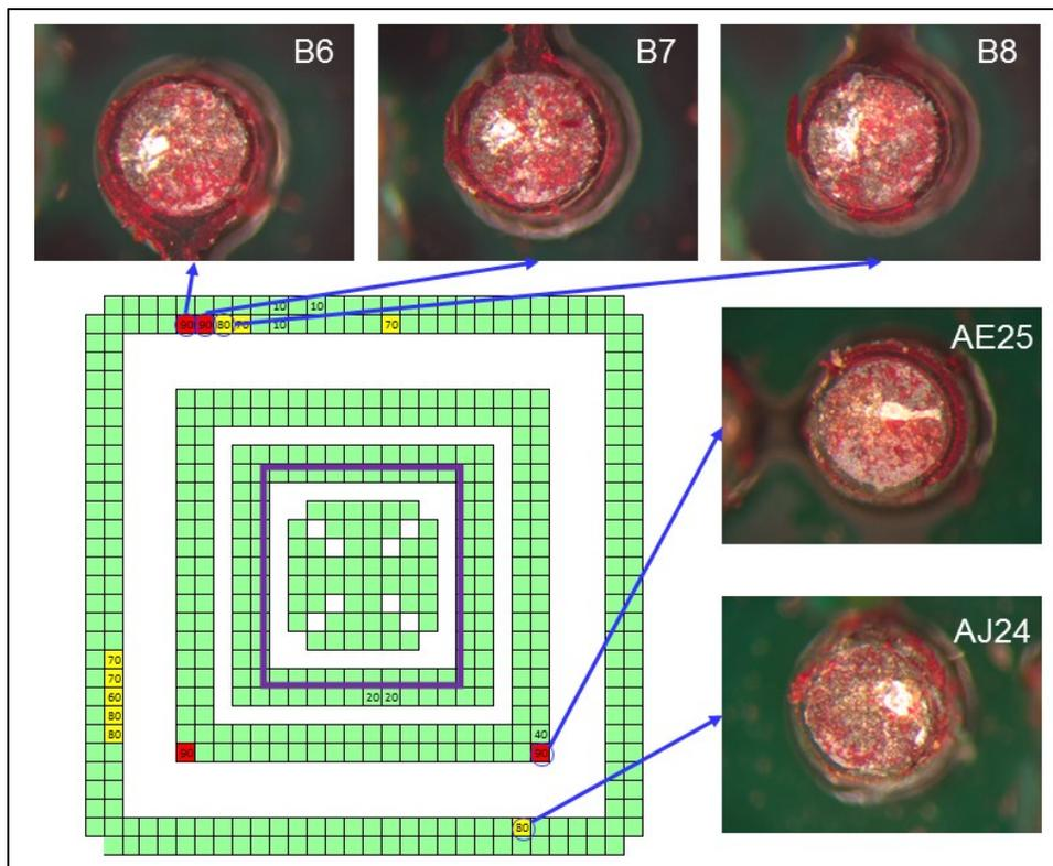
**Figure 16:** Example dye-and-pry results after 4013 cycles from Cell 1. Images are PCB view, on top of BGA ball attached to PCB pad after pry. Fracture surfaces were between solder ball and package BGA pad. Red area was fractured during cycling. Shiny area was still intact.
