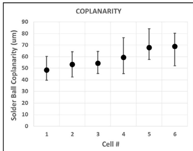
Figure 7: Solder ball coplanarity at room temperature.
