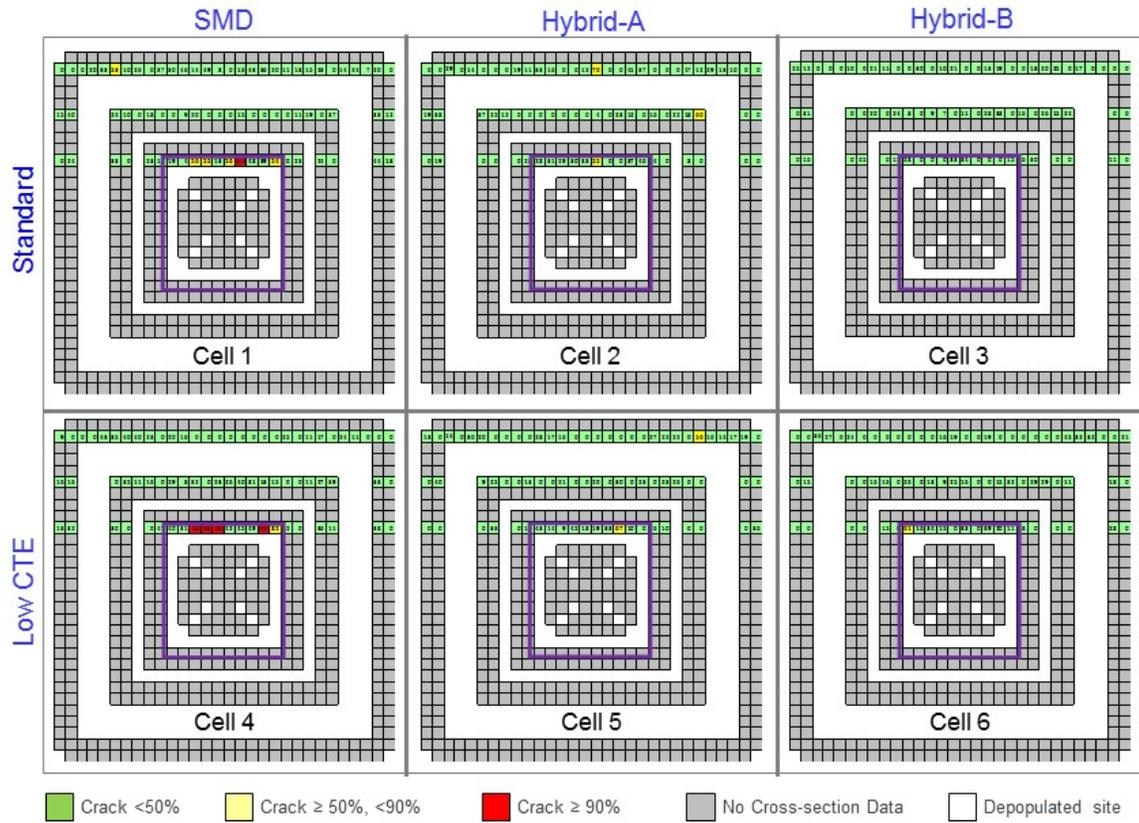
Figure 12: Distribution of degree of crack growth after 3000 cycle, as determined by cross-section.
