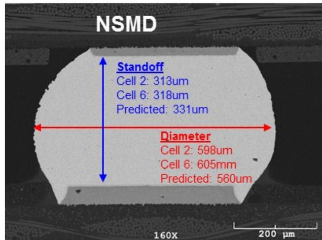
Figure 10: Cross-section of typical NSMD solder-joint after mounting to PCB.
