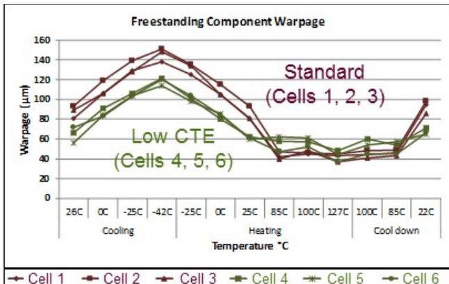
Figure 8: Package warpage by Thermoairé.
